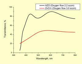
Figure 3. Transmittance of AZO and ZnO:Ir depending on the wavelength.
