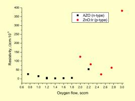
Figure 2. Resistivity of AZO and ZnO:Ir depenting on the oxygen gas flow.
