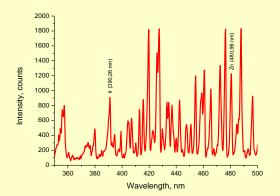
Figure 1. Optical emission spectrum upon sputtering of a metallic mosaic targets made of Zn and Ir pieces, with Zn=94%, Ir=6% surface area.
