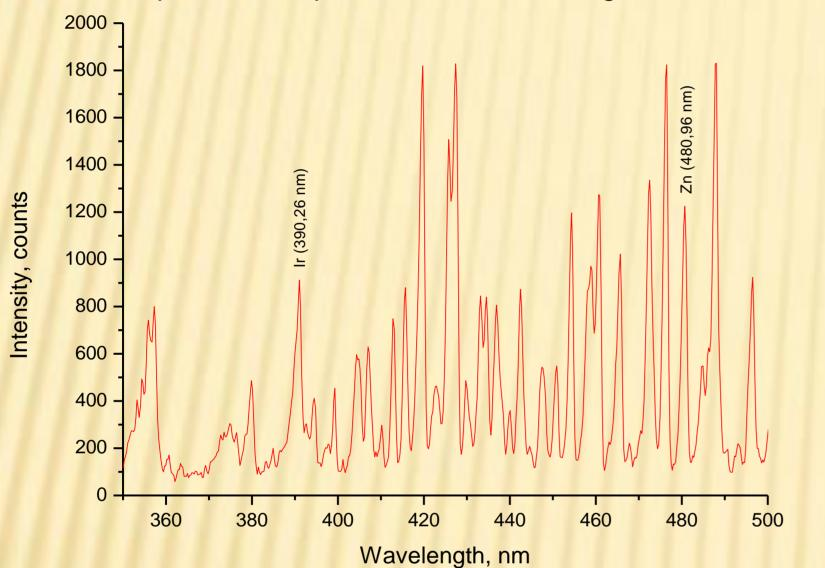
Fig.1. Plasma optical emission spectrum upon sputtering of a metallic mosaic target made of Zn and Ir segments with Zn 94%, Ir 6% surface area.
