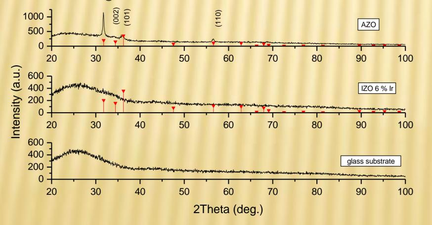
Fig.2. XRD spectra for the films of AZO (top), IrZO (middle) and a bare glass substrate (bottom).
